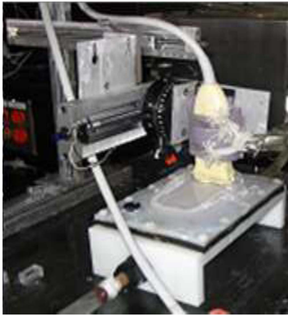
FIG. 3. Ultrasound probe fixed on a step motor to perform a linear scan in cross-sectional view of the vessel embedded within the phantom box.
