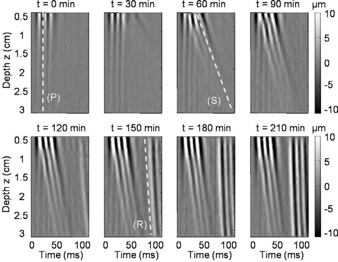
Fig. 2. Displacement field in an agar-gelatin mixture (3% agar and 2.5% gelatin) at different times (from 0 to 210 minutes) during the solidification process. The displacement field was plotted in gray color scale, along the depth  $z$  as a function of time. The low frequency pulse at 100 Hz was given at the time of 5 ms. Three different types of waves were noted: the bulk waves (P), the shear waves (S), and artificial secondary waves (R).
