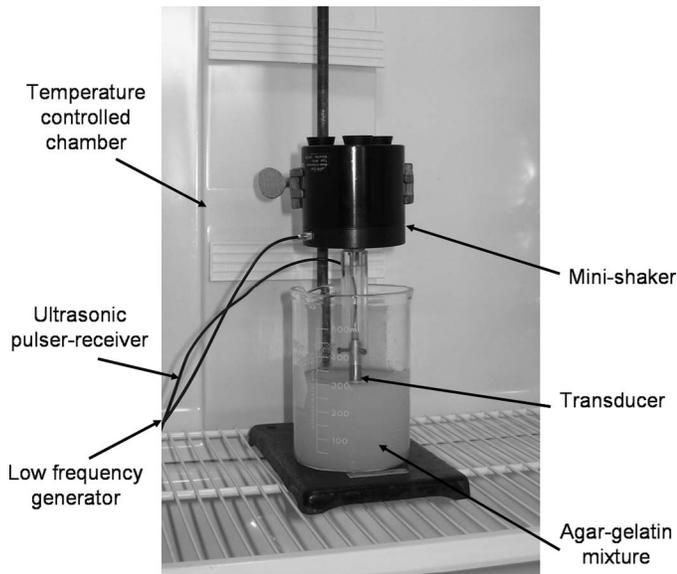
Fig. 1. Experimental setup, the shear elasticity probe was composed of a transducer mounted on a minishaker. The probe was placed in a temperature-controlled chamber at the surface of an agar-gelatin mixture in a liquid state. The gel solidification was followed for 12 hours.
