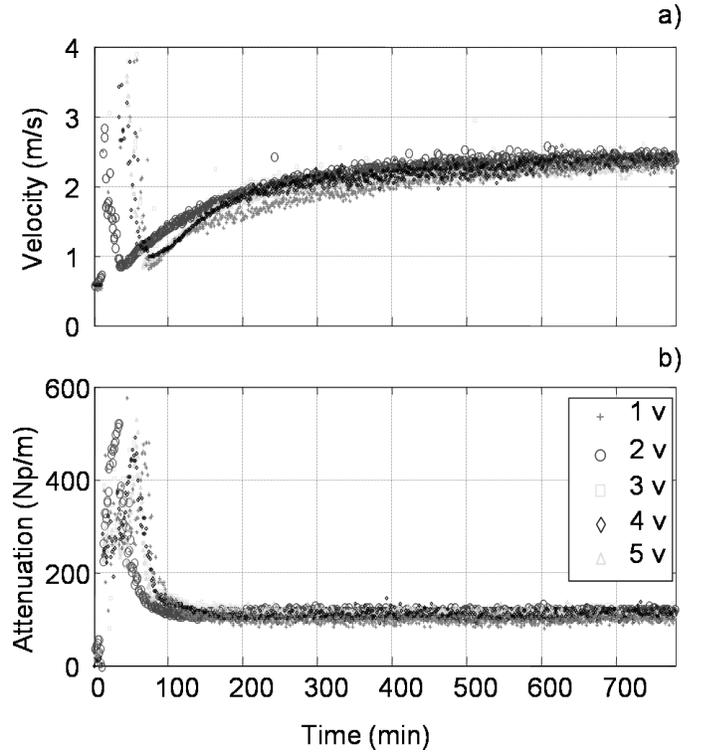
Fig. 5. Shear wave velocity (a) and shear wave attenuation (b) as a function of time for different amplitudes adjusted by the voltage on the minishaker (from 1 V to 5 V). The gelatin mixtures were composed of 3% agar and 3% gelatin. The shear wave frequency was set to 100 Hz.
