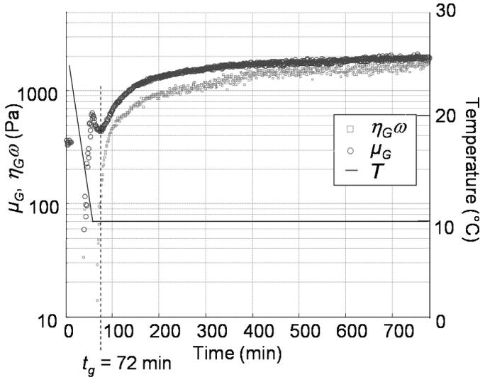
Fig. 7. Kinetics of gelation: relative elasticity  $\mu_G$  and relative viscosity  $\eta_G$  versus time at 100 Hz for an agar-gelatin mixture of 2.5% gelatin and 3% agar. The shear wave amplitude was adjusted by the minishaker voltage to 4 V.
