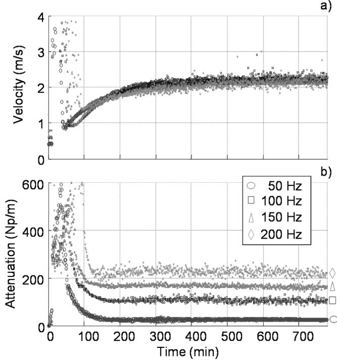
Fig. 3. Shear wave velocity (a) and shear wave attenuation (b) as a function of time for different frequencies (from 50 Hz to 200 Hz). The gelatin mixtures for these four experiments were composed of 3% agar and 3% gelatin. The shear wave amplitude was adjusted by the minishaker voltage that was set to 4 V.
