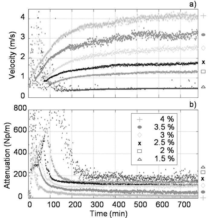
Fig. 6. Evolution of the shear wave velocity (a) and shear wave attenuation (b) at 100 Hz as a function of time for different gelatin concentrations (from 1.5% to 4%). The shear wave amplitude was constant in those measurements (the minishaker voltage was adjusted to 4 V).
