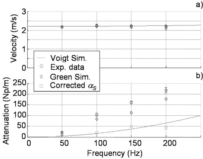
Fig. 4. Theoretical and experimental shear wave velocities (a) and shear attenuations (b) as a function of frequency. The experimental data for attenuation ( $\circ$ ) was corrected with a Green's function simulation ( $\diamond$ ) to compensate for the diffraction effects. The corrected attenuation  $\alpha_S$  values ( $\square$ ) were in good agreement with the theoretical predictions (solid line).
