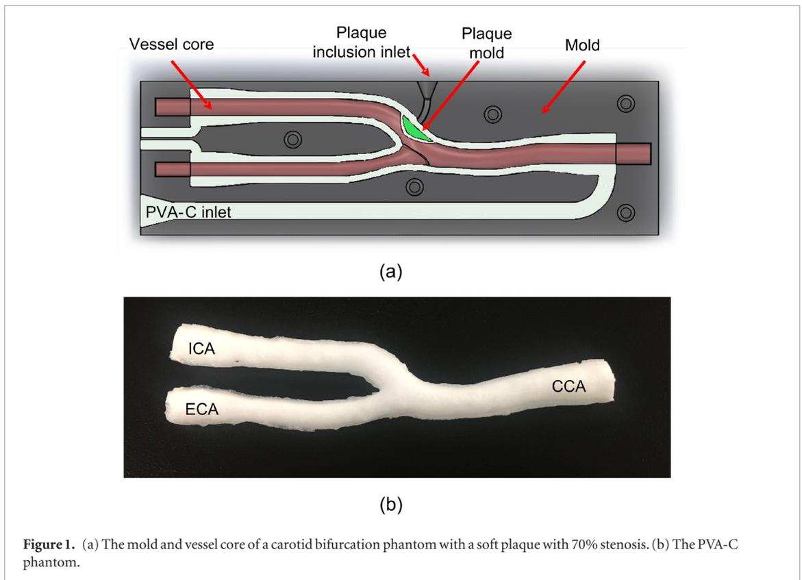
**Figure 1.** (a) The mold and vessel core of a carotid bifurcation phantom with a soft plaque with 70% stenosis. (b) The PVA-C phantom.
