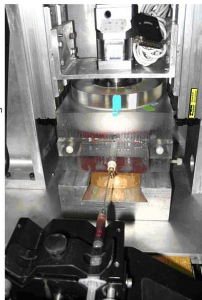
Fig. 1. Experimental Couette flow device (schematic view on the left, picture on the right).
