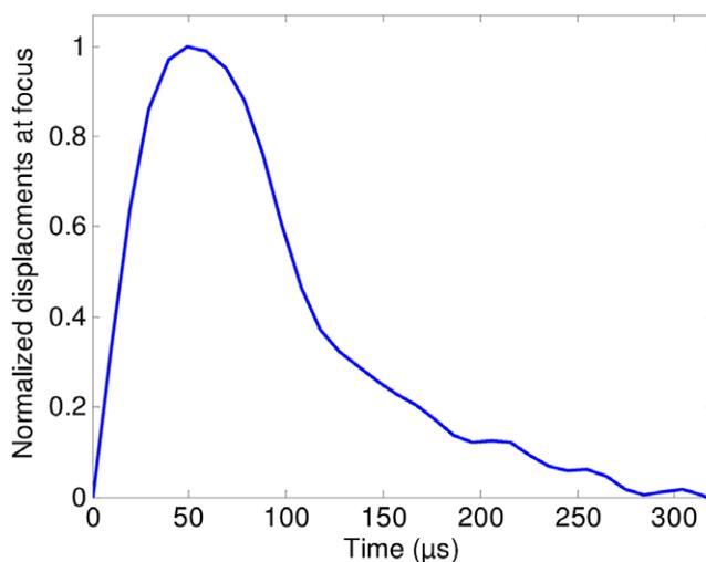
**Figure 6.** Normalized temporal displacement at the focus of the transient excitation.
