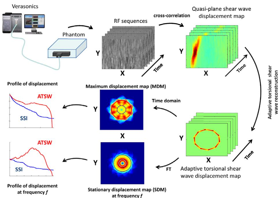
**Figure 1.** Schematic illustration of the experimental setup and data post-processing.
