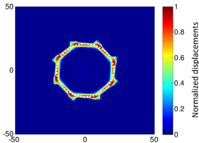
**Figure 2.** Schematic illustration of the combination of the eight quasi-plane wavefronts around a closed path (dashed white circle) to generate the adaptive torsional shear wave (ATSW). The color scale from blue (minimum), green and red (maximum) indicates the amplitude of normalized displacements.  $X$  and  $Y$  distances are in mm.
