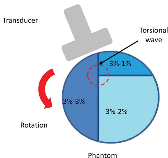
**Figure 3.** Schematic representation of the complex heterogeneous phantom #6. Torsional shear waves were generated around an eccentric closed circular path by moving the position of the transducer. Percentages represent proportions of agar and gelatin.
