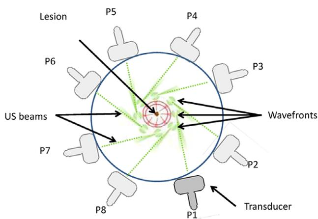
**Figure 4.** Schematic representation of the mechanical rotation of the ultrasound transducer around the phantom from position 1 (P1) to position 8 (P8).
