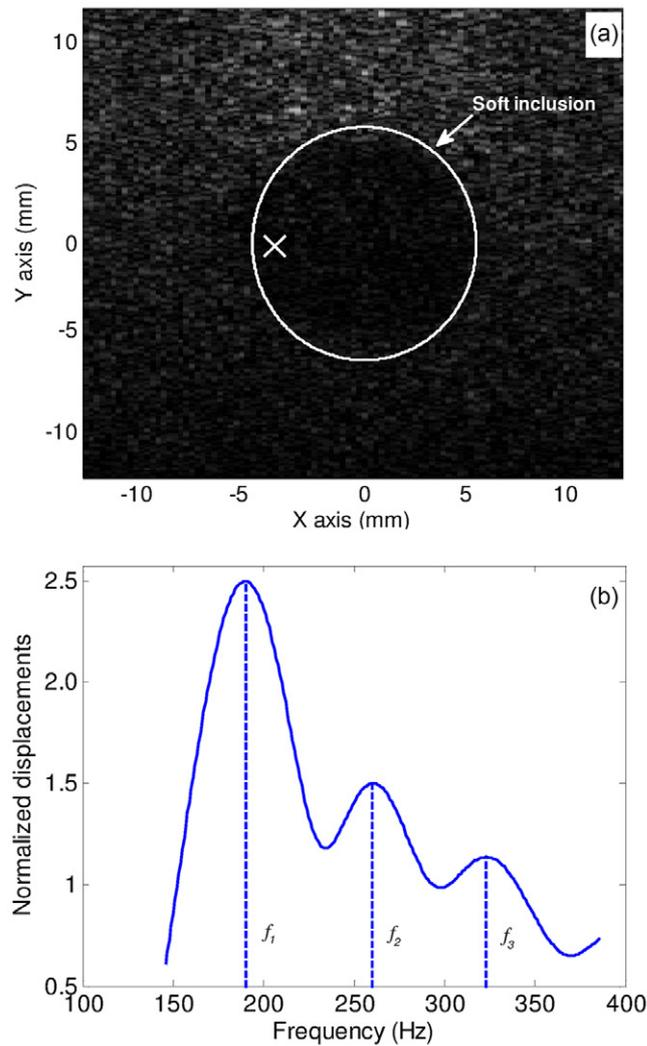
**Figure 13.** (a) B-mode image of the heterogeneous phantom #4 with a soft inclusion. The white cross within the soft inclusion represents the displacement spectrum measurement site  $M$  ( $-4, 0$  mm). (b) Normalized displacement spectrum within the soft inclusion with respect to the focus push.
