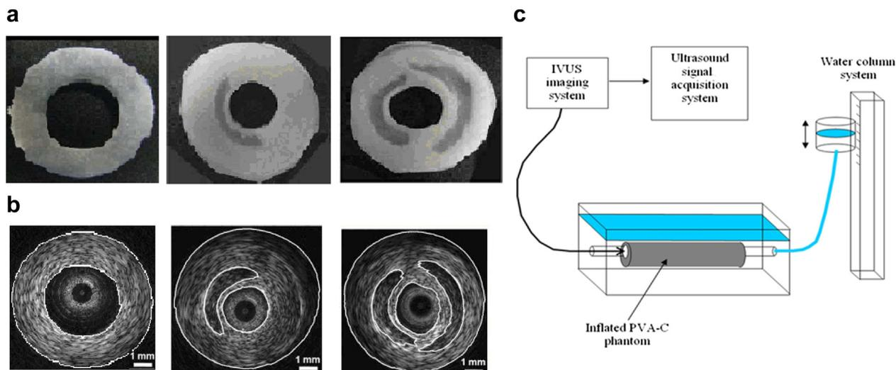
Fig. 1. (a) Sections of two polyvinyl alcohol cryogel (PVA-C) phantoms. (b) Corresponding B-mode intravascular ultrasound (IVUS) images. (c) Diagram of the experimental setup comprising a water tank, the PVA-C phantom, a water column system to pressurize the phantom and the ultrasound acquisition system.
