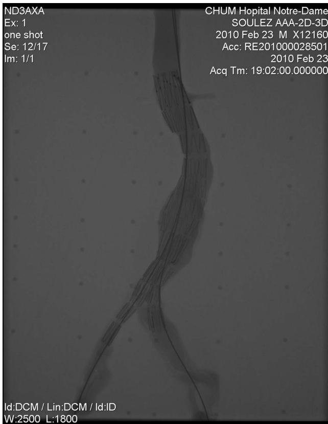
FIG. 7. CTA image showing a stent graft deployed into the lumen of the AAA phantom and a visible thrombus. Fiducial markers are seen in the background of the image.
