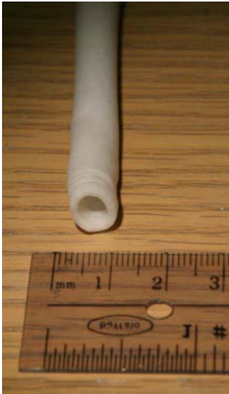
FIG. 1. Picture of the PVA-made vessel-mimicking phantom.
